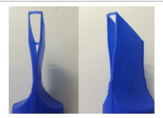
In the procedure before the Federal Patent Court, the dispute focused on the question of whether the two plastic strips of the Defendant's valve as shown above are sufficiently "separate" from each other as claimed by feature 1.3 of claim 1.
